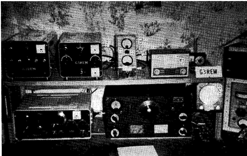
G3REM is operated by John Austin at 40 Cross Keys, Bearsted, Maidstone, Kent. Licensed in August 1962, he has a pretty comprehensive layout. At lower left is a Sphinx three-band SSB Tx and then an HRO with some useful modifications. After the bug-key and at extreme right is a Gelo rig. On the upper shelf, to the left, is a home-built TT21 linear and its 1250v. solid-state PSU, to match the Sphinx, then an aerial control panel, and the invaluable Heathkit SWR bridge, with an RF monitor unit behind. G3REM served in the R.A.F. during 1937-'46, flying in aircraft carrying the (then) battery-type Tx/Rx gear, and one of his Squadron's routine jobs was target-towing for the Royal Navy—so John learnt his CW by having to use "blinker" with an Aldis lamp! (Well, it's one way of getting the Morse!)
