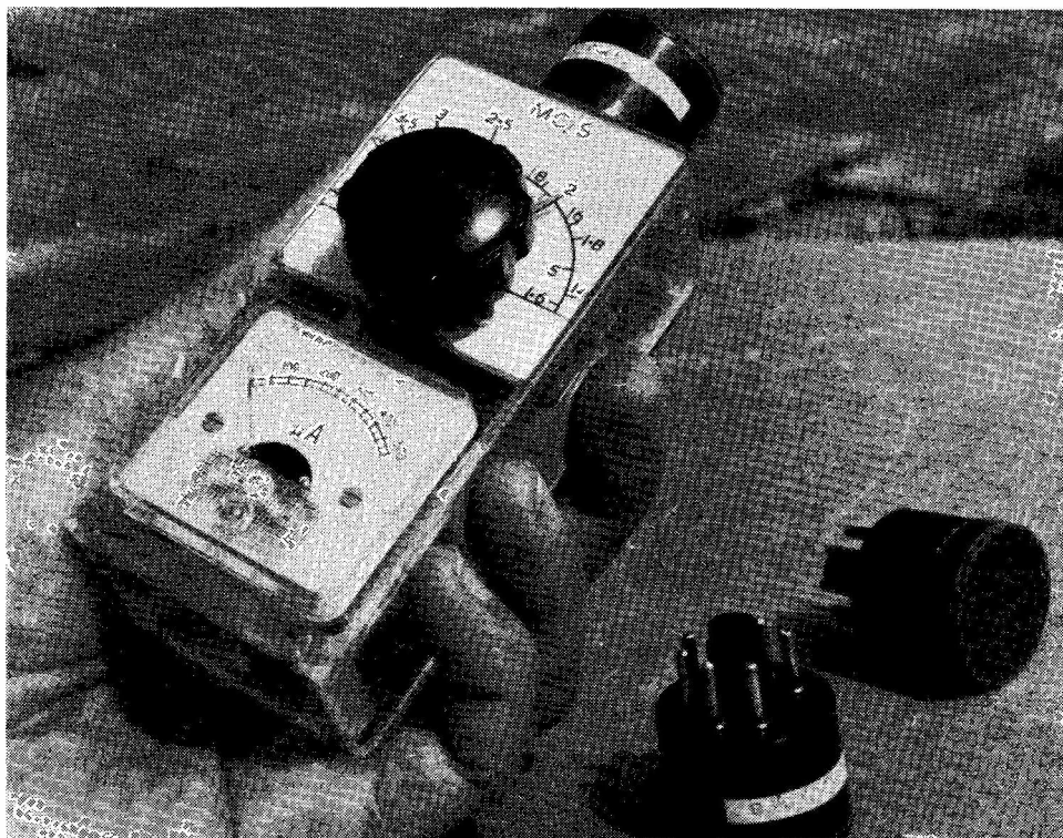
The instrument described in the article by G3OGR. It is in effect a calibrated wavemeter, with meter indication. If carefully used and calibrated with reasonable care (see text) it will be found invaluable for a number of checking functions on transmitter circuits. The meter-and-diode takes the place of the loop-and-lamp on the earlier and more conventional type of direct-reading wavemeter.
